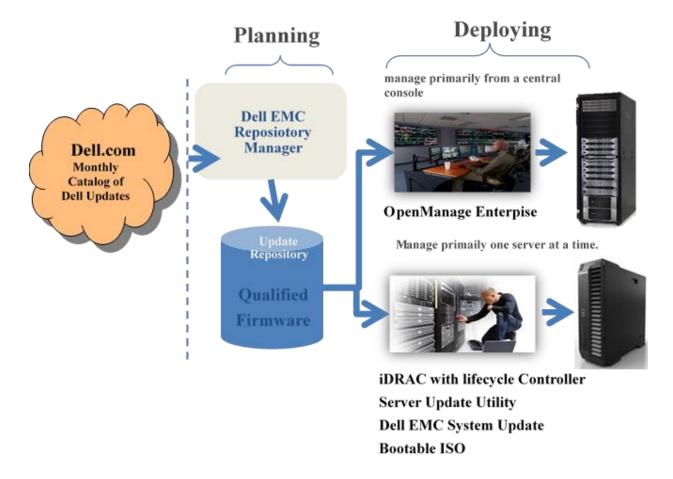
Figure 1 Planning and Deployment phases in updating the Dell EMC Enterprise Systems Applications
