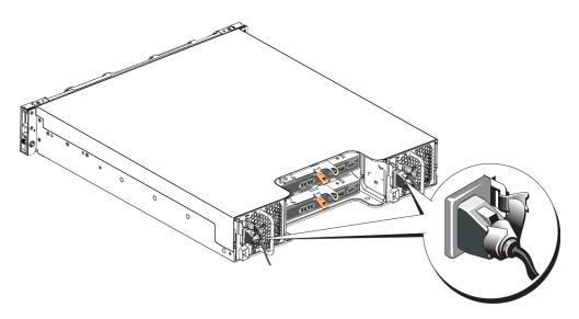
Figure 35: Securing the Power Cables (1080W Power Supply)
