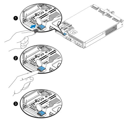
Figure 23: Inserting the MicroSD Card
