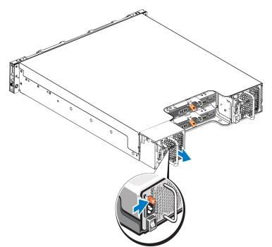
Figure 30: Removing a 700W Power Supply and Cooling Module
