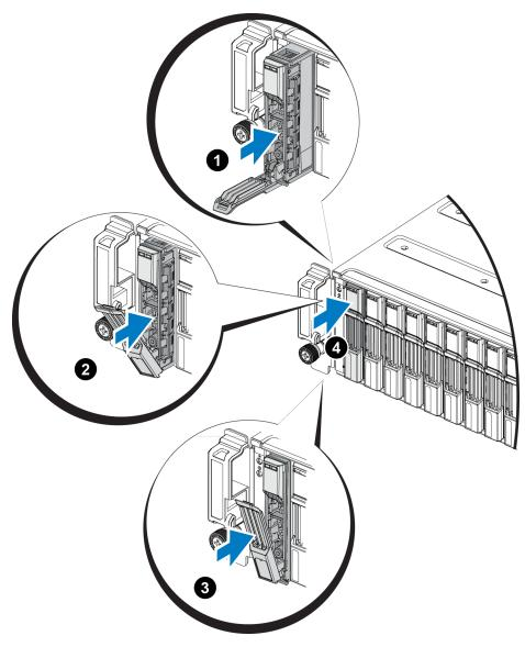
Verify that the new drive is operational by examining the LEDs on the front panel, as described in *Interpreting Drive LEDs on page 7*. In addition, examine the GUI Member Disks window and the CLI member select show disks command output.
