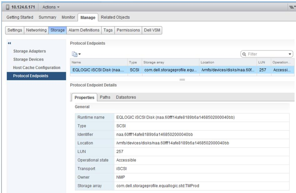
Figure 14 Protocol endpoint as shown in vSphere Web Client
