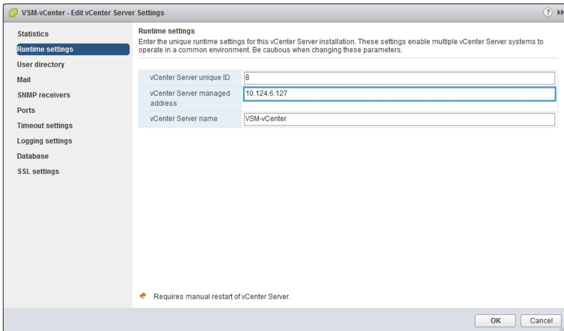
Figure 1 Setting vCenter Server managed address
