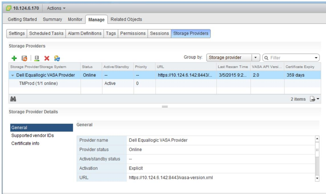
Figure 3 Listing of vSphere Storage Providers – vSphere 6.0 example
