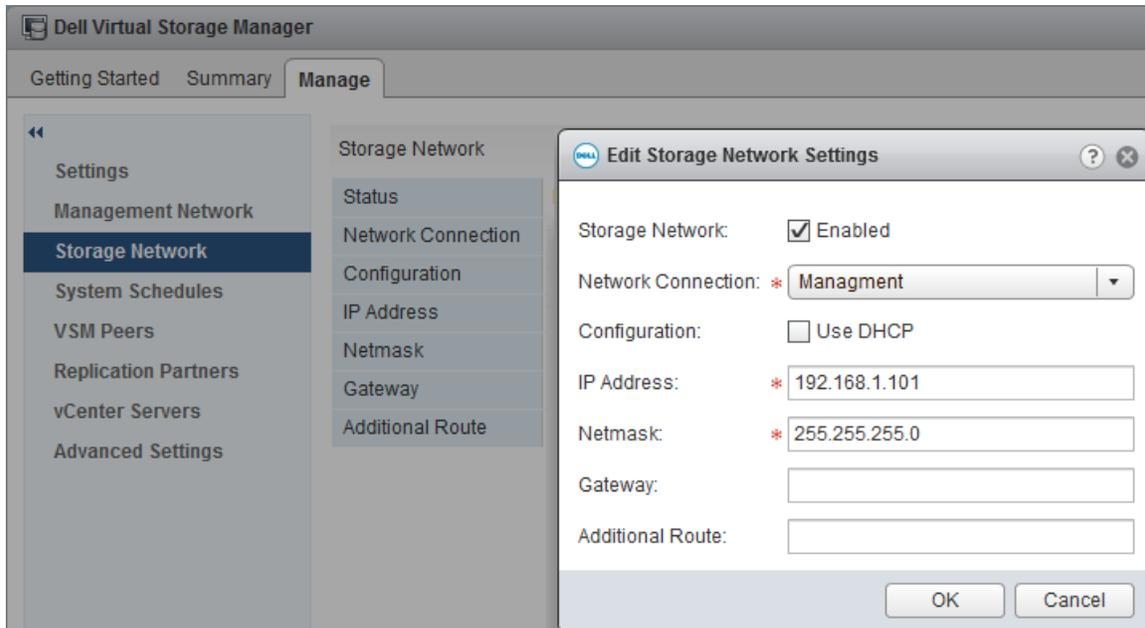
Figure 4 Configuring the optional Storage Network in VSM 4.0
