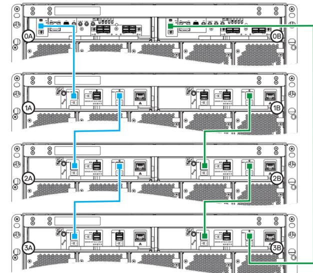
Figure 6. 5U dual-controller cabling (reverse method)
