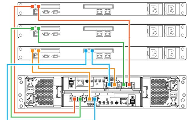
Figure 13. 2U direct attached SAS host server connections
