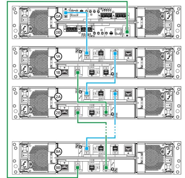
Figure 5. 2U dual-controller cabling: maximum 10 enclosures (reverse method)
