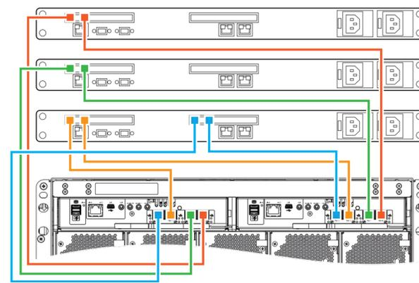
Figure 14. 5U direct attached SAS host server connections
