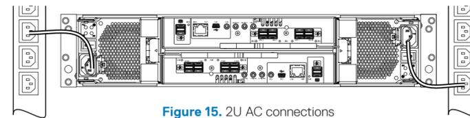
Figure 15. 2U AC connections
