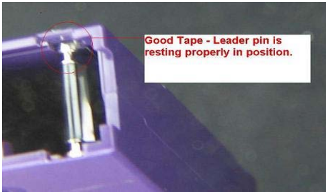
Figure 1-6. Media Inspection - Good Tape
