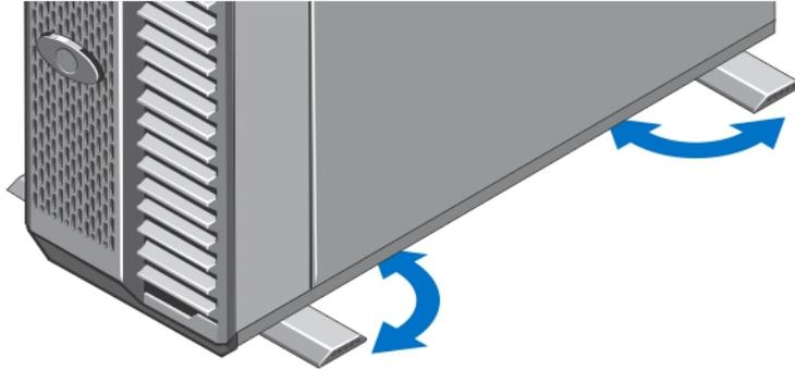
Figure 2. Extending the Feet of the Tower System
