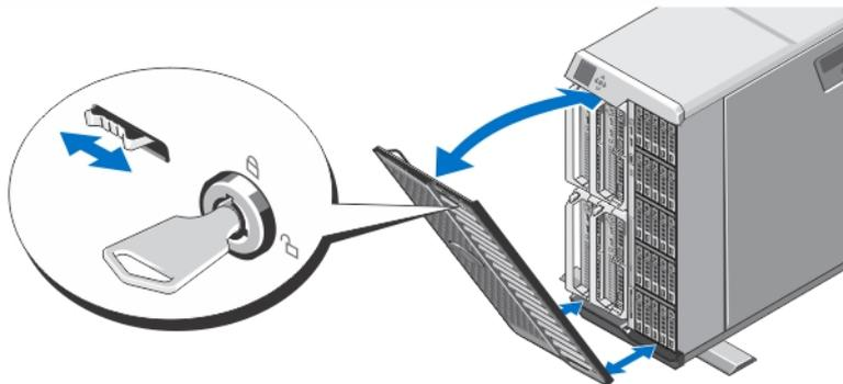
**Figure 11. Installing the Optional Bezel**
