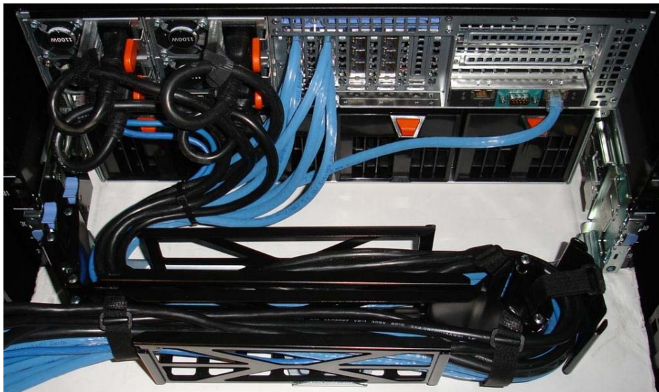
Figure 5. Right-side mounted CMA installation
