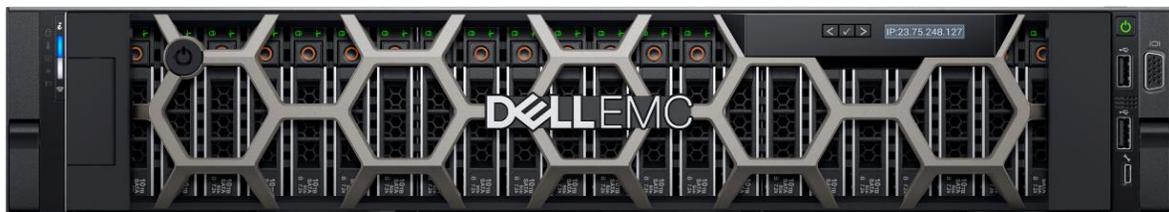
Figure 5 Dell EMC PowerEdge R740xd server
