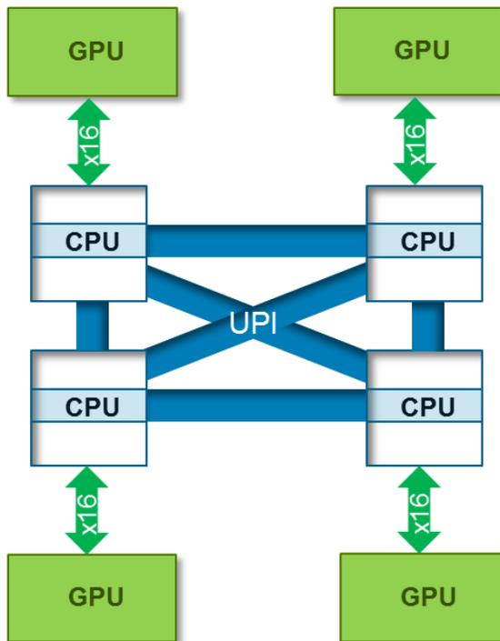
Figure 7 PowerEdge R940xa GPU Topology
