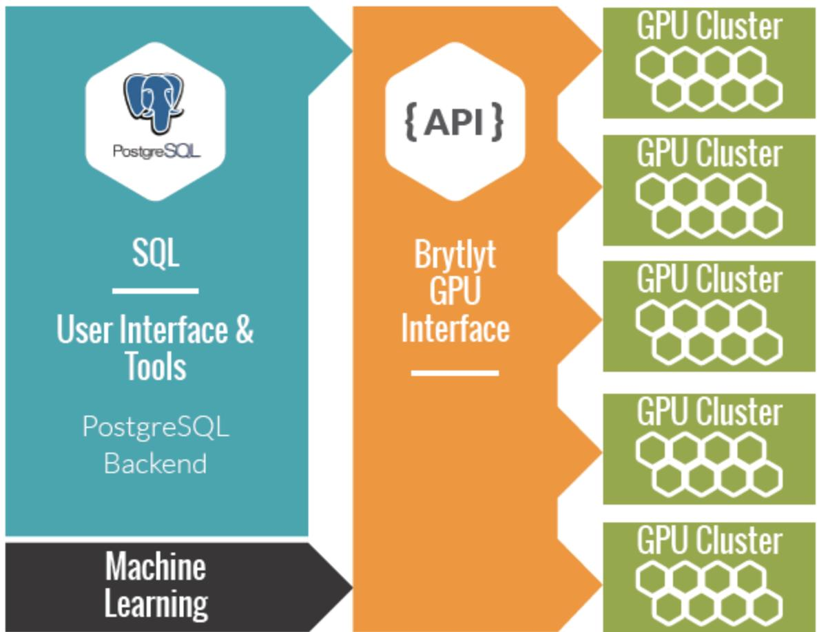
Figure 3 Block Diagram of Brytlyt stack interfacing between PostgreSQL and GPU Cluster
