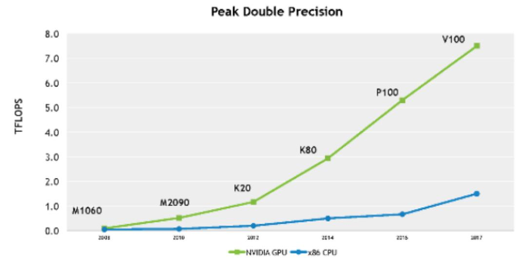
Figure 2 GPU Flop Comparison vs. CPU [source: NVIDIA]
