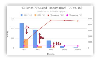
blocks to simplify deployment and speed scaling with unmatched performance. To increase performance, customers simply need to move their network from 1Gb to 10Gb thus increasing throughput and storage IOPS. The move to 10/25Gb Ethernet speeds translates to increased application performance along with better utilization and scaling of existing compute power and storage performance. This testing is clear that vSAN deployments would significantly benefit from upgrading from 1Gb to 10/25Gb speed
