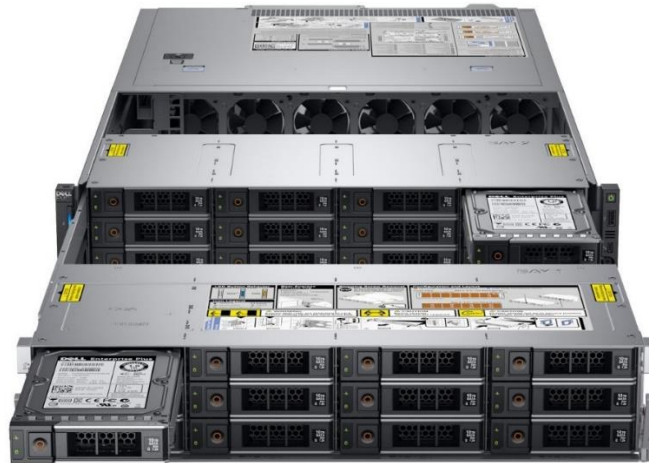
Image 2: PowerEdge R740xd2 with chassis expanded, permitting easy access to all drive bays.
