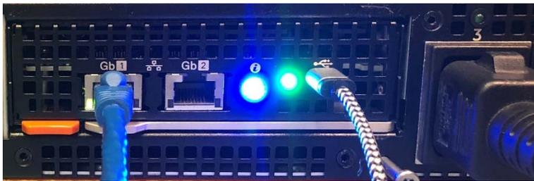
Figure 10 Solid Blue LED at the rear of the chassis
