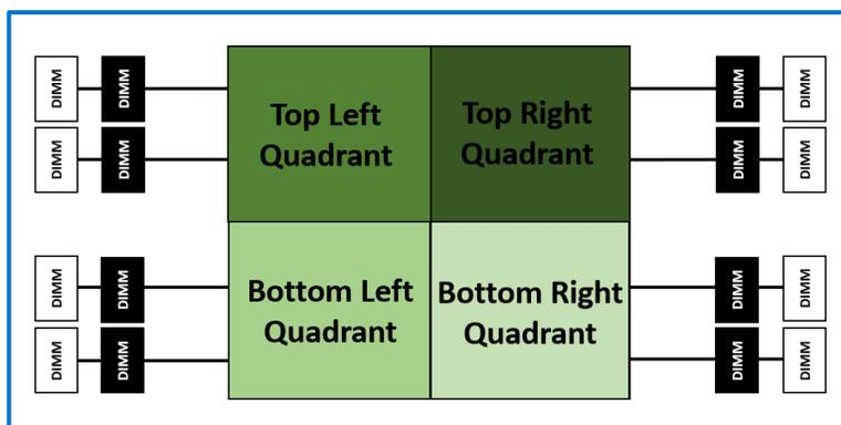
Figure 2: Quadrant layout of Rome processors
