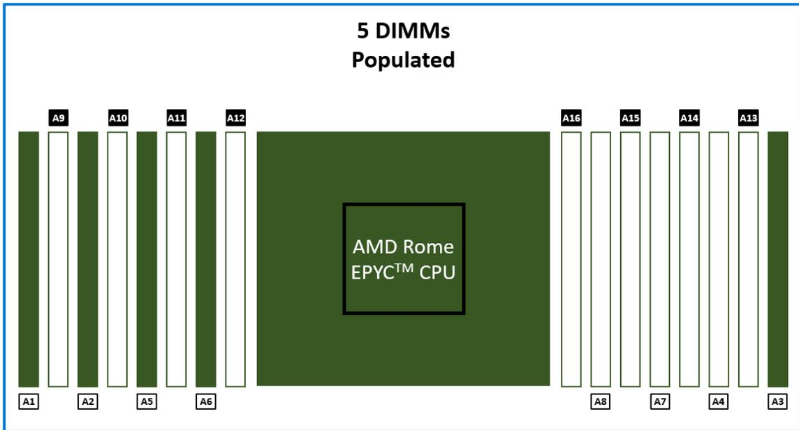
Figure 15: Five DIMMs are populated in an unbalanced configuration
