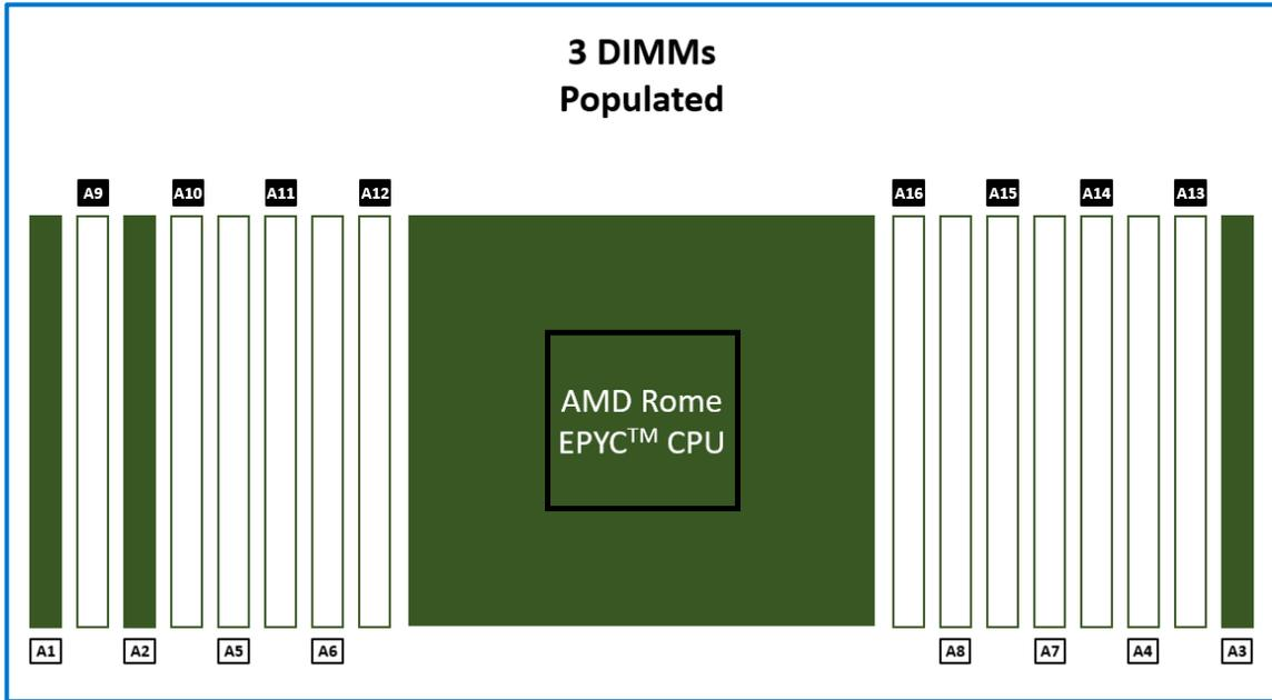
Figure 14: Three DIMMs are populated in an unbalanced configuration
