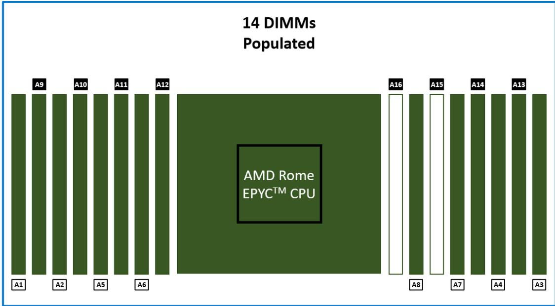
Figure 22: Fourteen DIMMs are populated in a near balanced configuration
