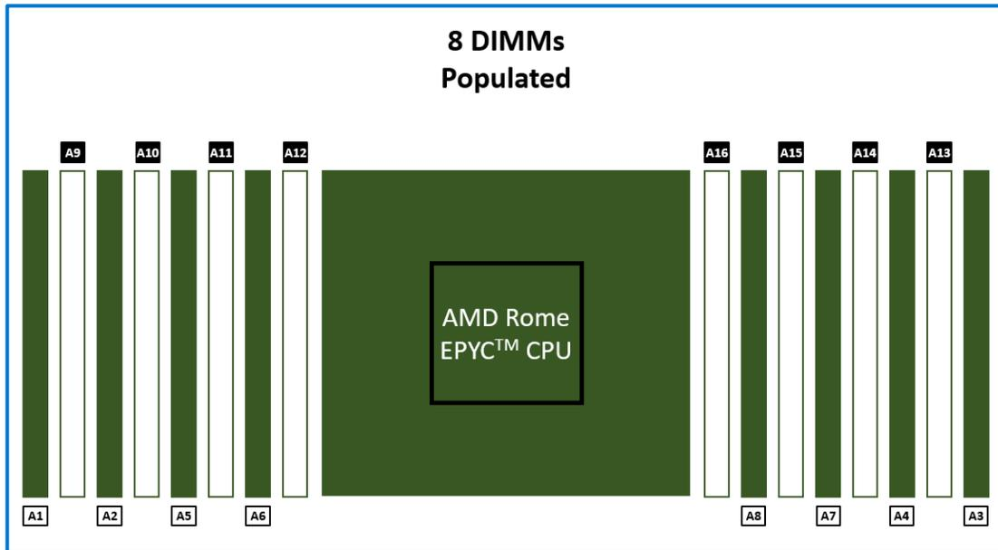
Figure 8: Eight DIMMs are populated in a balanced configuration, producing the highest memory bandwidth while at a lower capacity than sixteen
