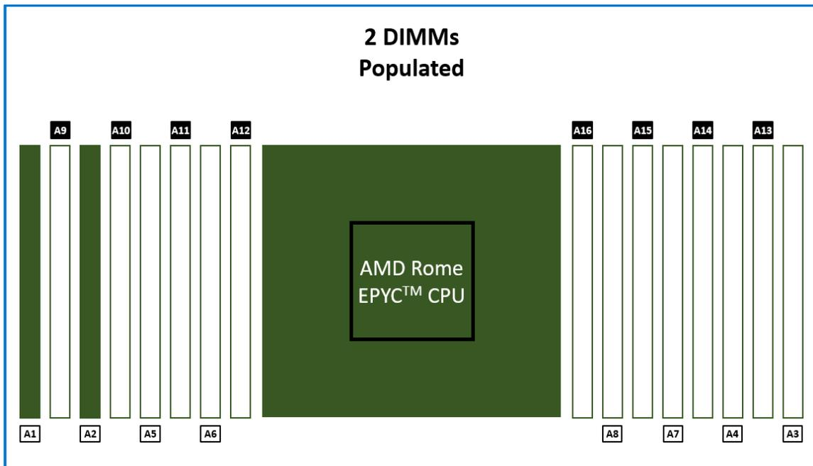
Figure 13: Two DIMMs are populated in an unbalanced configuration
