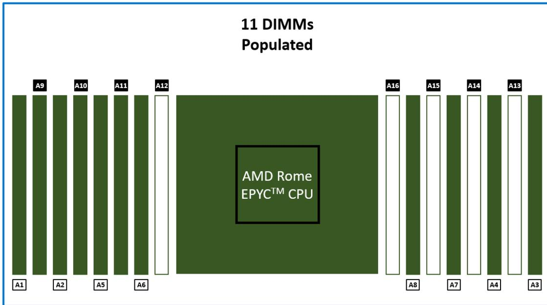
Figure 20: Eleven DIMMs are populated in an unbalanced configuration
