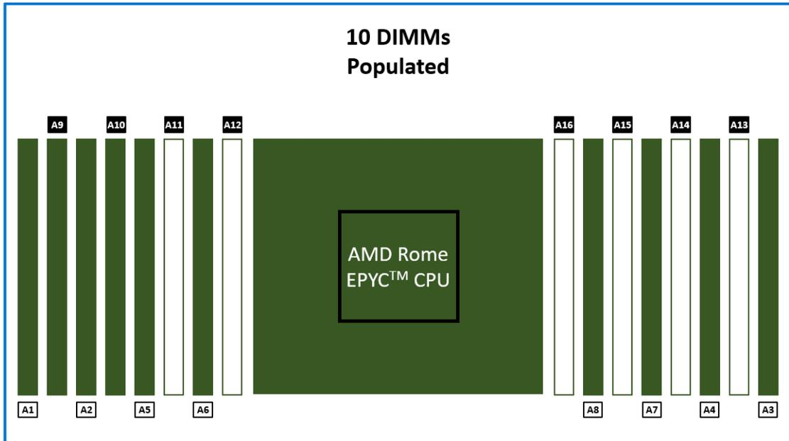
Figure 19: Ten DIMMs are populated in a near balanced configuration
