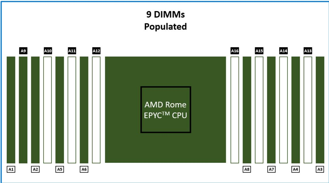
Figure 18: Nine DIMMs are populated in an unbalanced configuration
