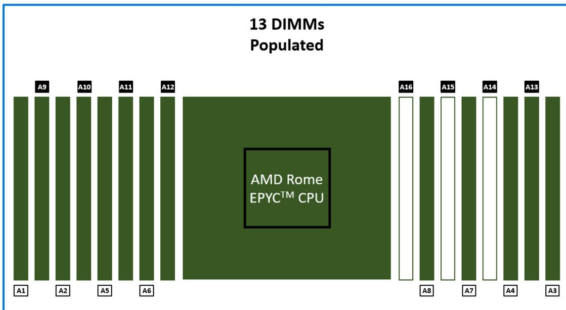
Figure 21: Thirteen DIMMs are populated in an unbalanced configuration
