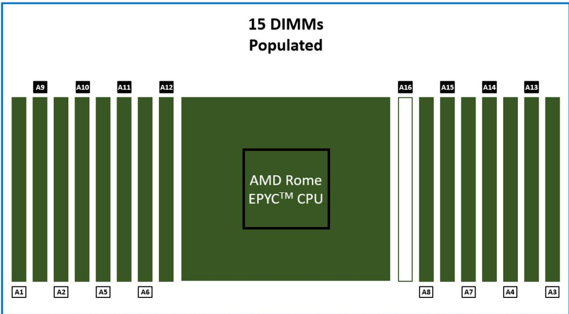
Figure 23: Fifteen DIMMs are populated in an unbalanced configuration
