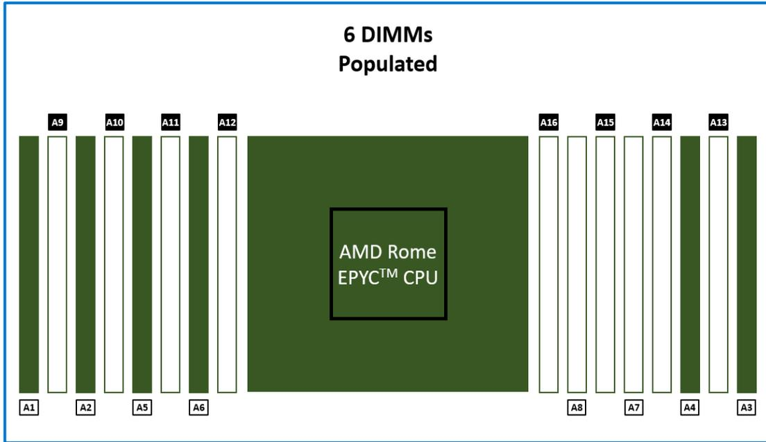
Figure 16: Six DIMMs are populated in a near balanced configuration
