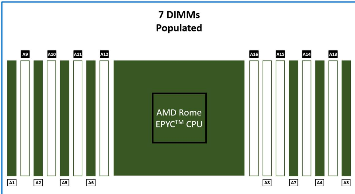
Figure 17: Seven DIMMs are populated in an unbalanced configuration
