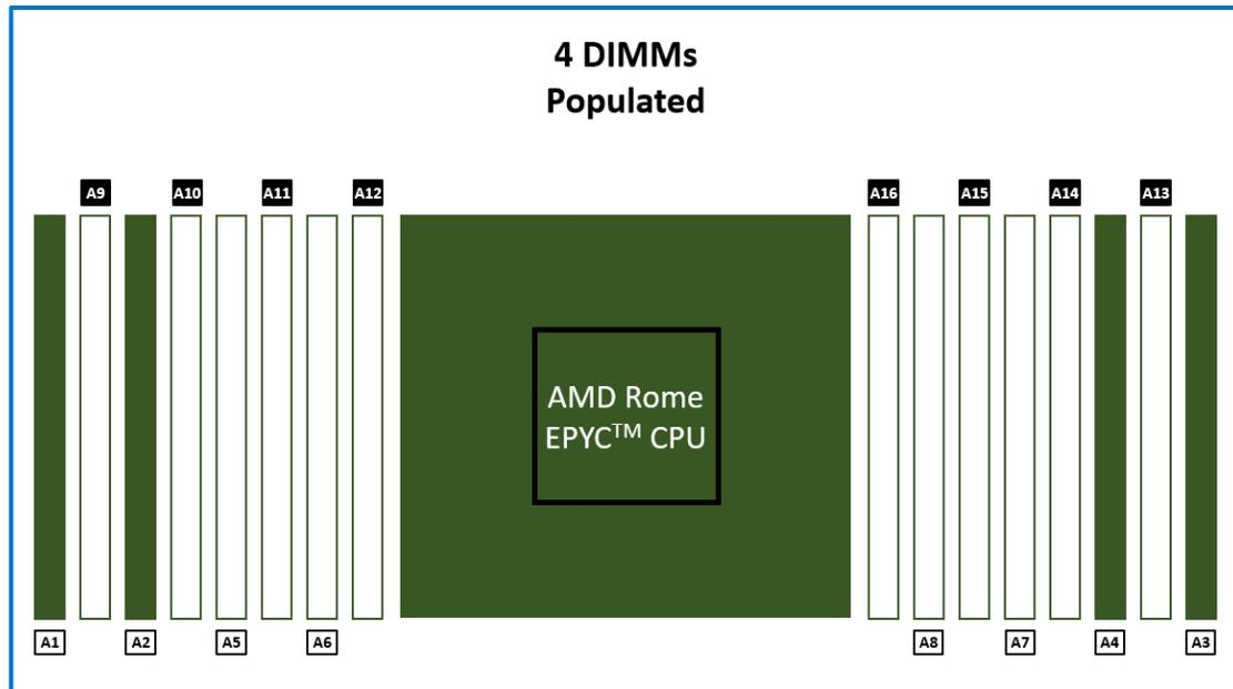
Figure 10: Four DIMMs are populated in a near balanced configuration
