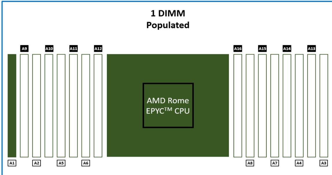
Figure 12: One DIMM is populated in an unbalanced configuration
