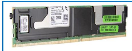
Figure 1: The 8Rx4 PC4-2666V DCPMM has a DRAM form factor but functions as both a memory and storage technology
