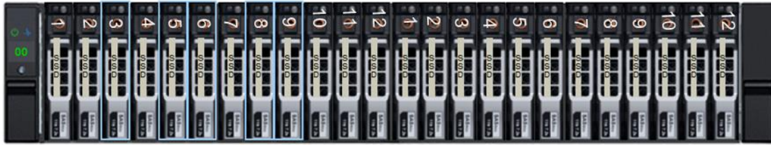
Figure 6 ME4024 drives assigned to LUN for Configuration with High Demand Meta Data.
