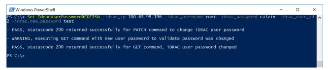
Figure 6 Changing iDRAC user password with set-IdracUserPasswordRedfish cmdlet
