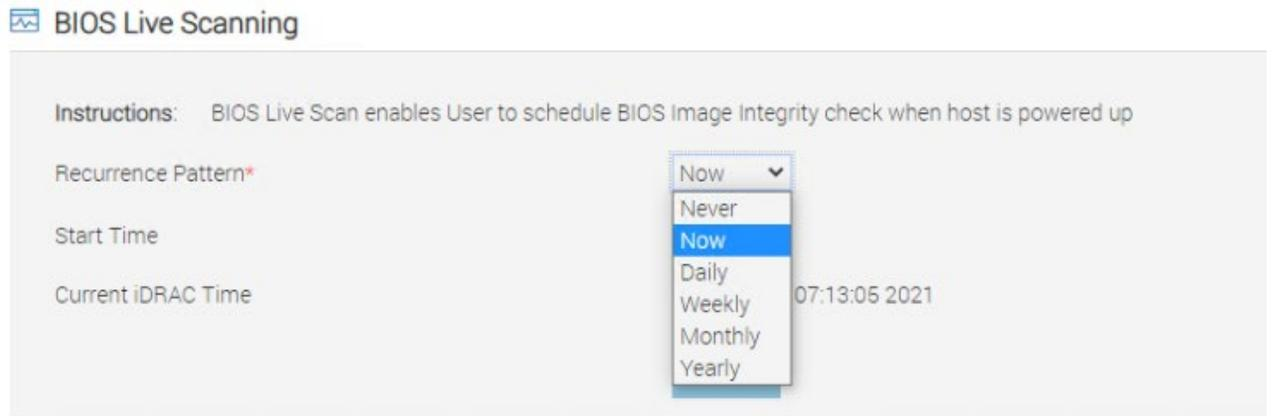
Figure 3 BIOS live scanning options in iDRAC UI.
