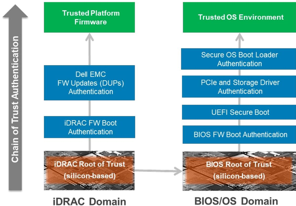
Figure 1 Silicon-based Root of Trust Domains in PowerEdge Servers with iDRAC9.
