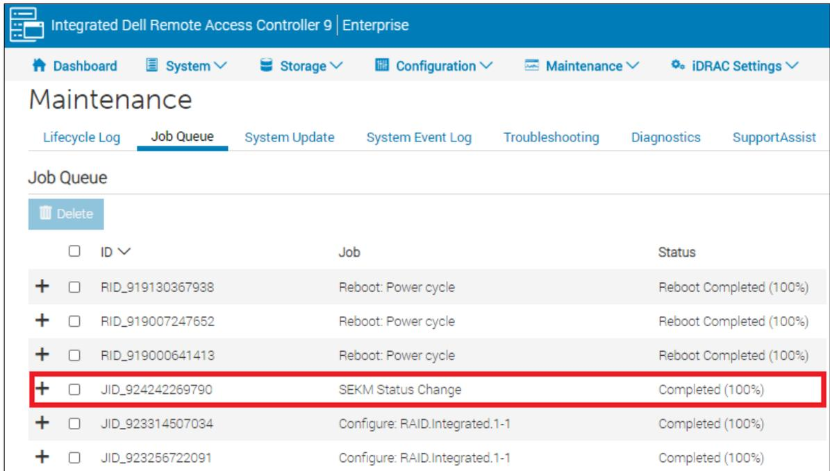
Figure 34 A job to enable SEKM is successfully completed
