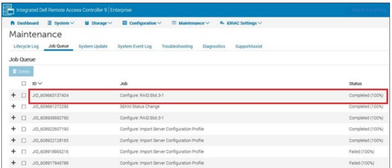
Figure 18 A job successfully run to enable SEKM on iDRAC PERC
