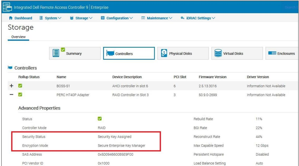
Figure 19 Ensure that SEKM is enabled on your controller
