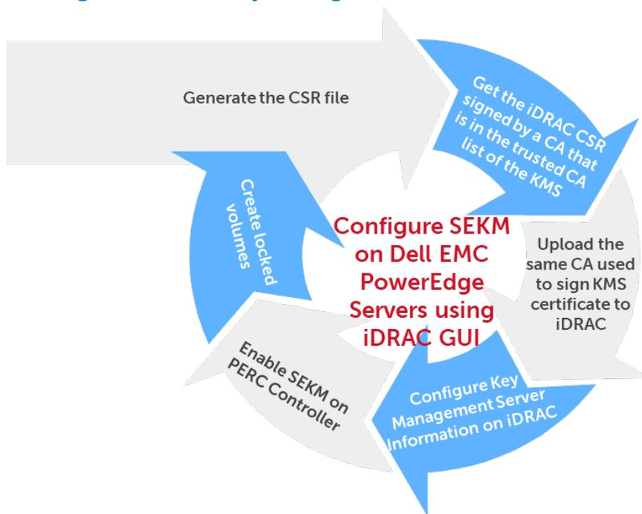
Figure 3 Key processes in configuring SEKM on PowerEdge servers by using iDRAC GUI
