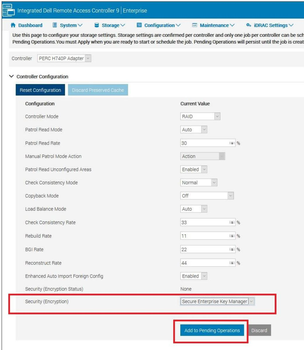
Figure 15 Enable SEKM on iDRAC PERC
