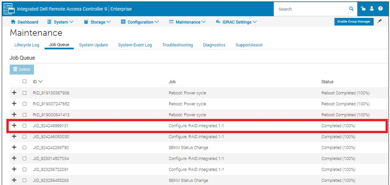
Figure 37 A job successfully ran to enable SEKM on iDRAC PERC
