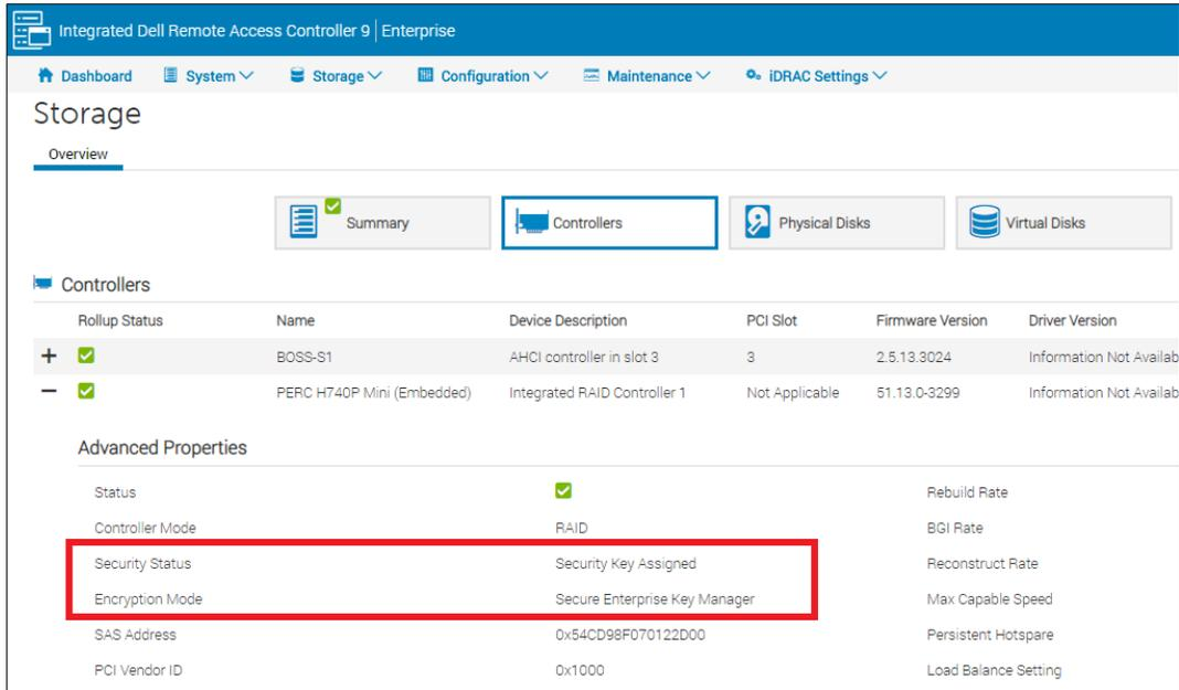
Figure 38 Ensure that SEKM is enabled on your controller
