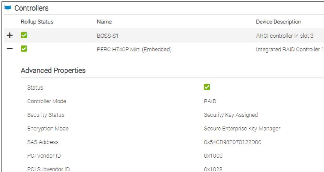
Figure 72 Ensure SEKM is enabled on iDRAC PERC
