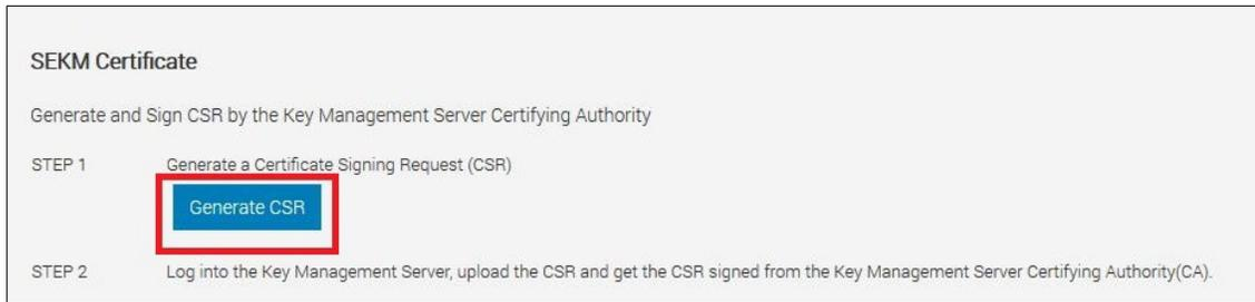
Figure 4 Generate CSR by using the iDRAC GUI
