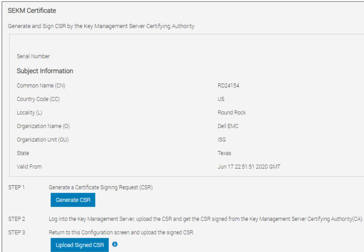
Figure 25 Upload the signed CSR certificate on iDRAC GUI
