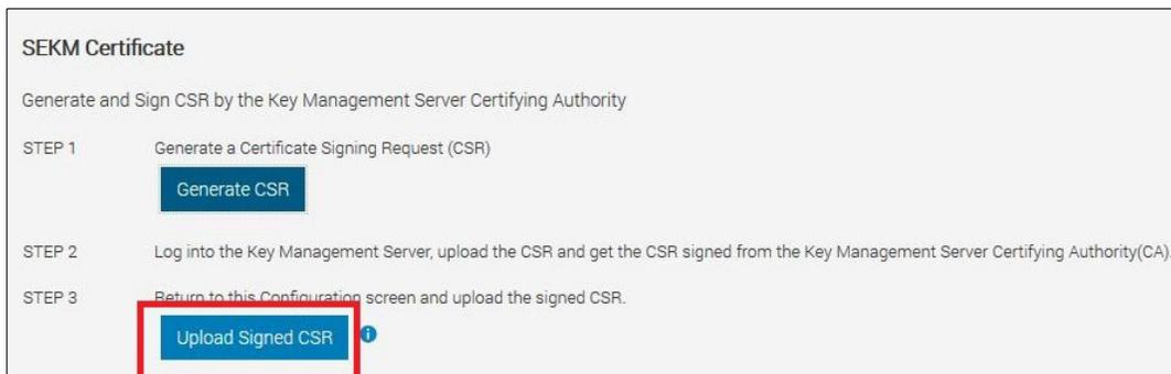
Figure 9 Upload the signed CSR certificate by using iDRAC GUI
