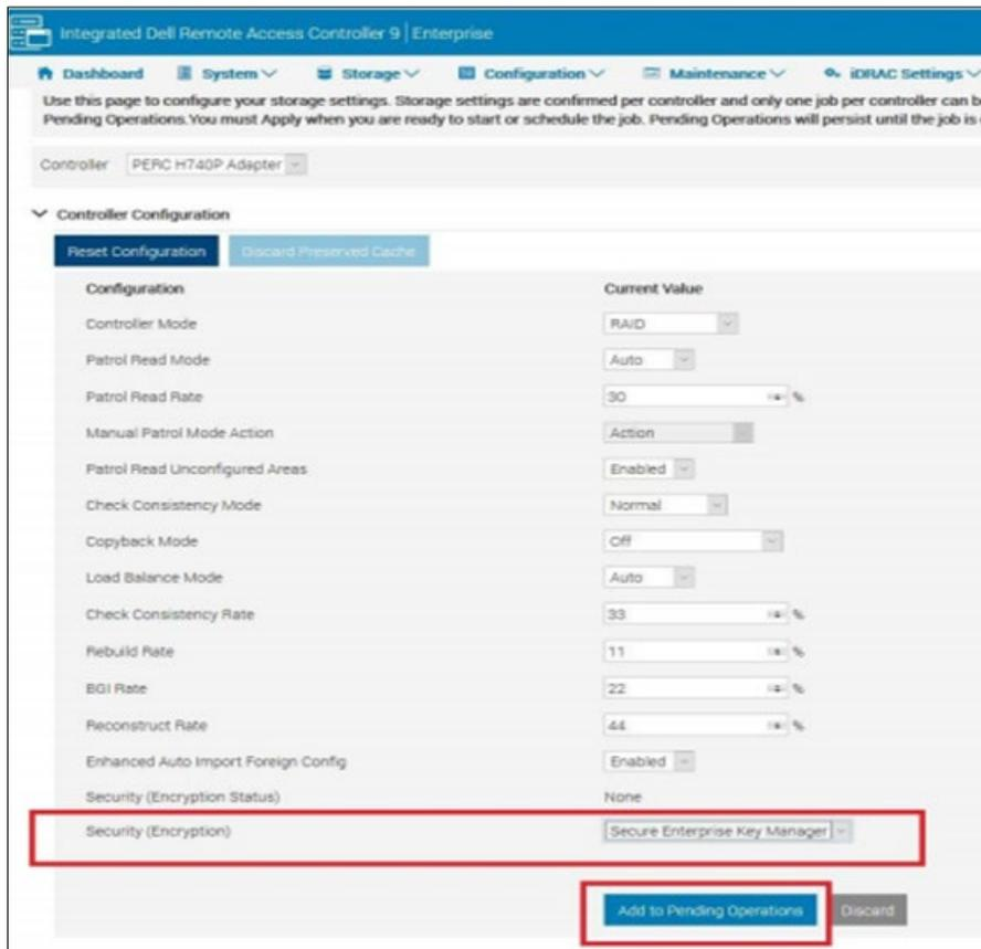
Figure 35 Enable SEKM on iDRAC PERC
