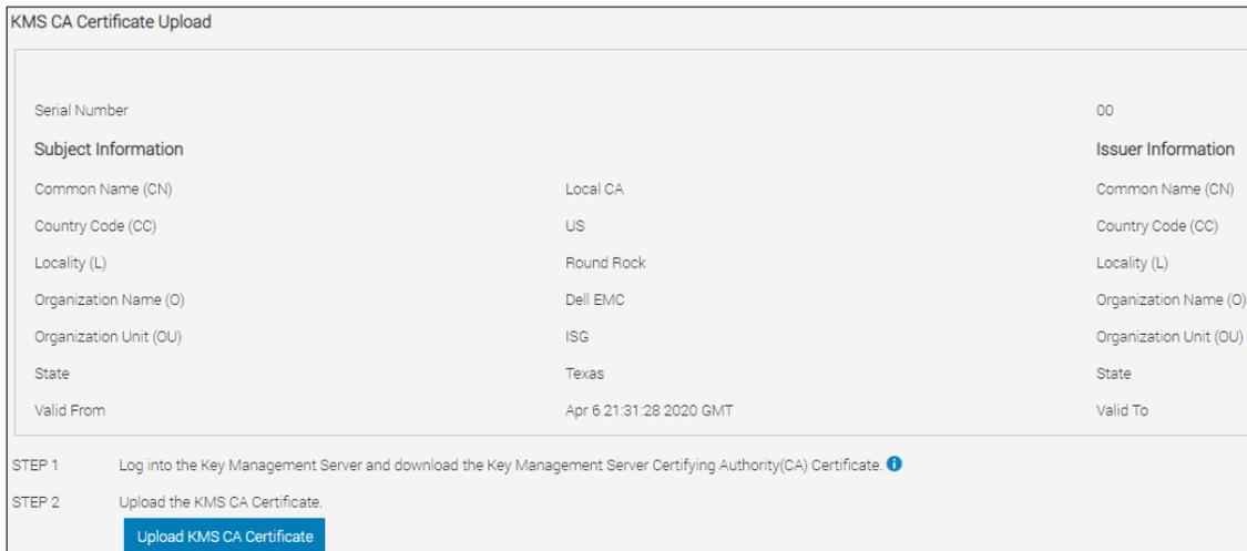
Figure 65 Upload KMS CA certificate to iDRAC
