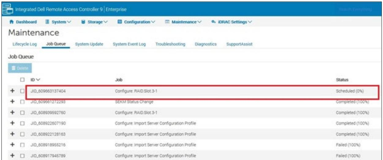
Figure 17 A job is scheduled to enable SEKM on iDRAC PERC
