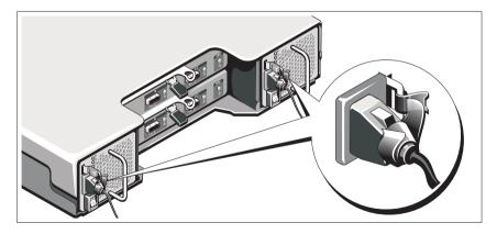
1 Bend the power cables as shown in the illustration and secure the cables firmly to the bracket using the strap provided.
