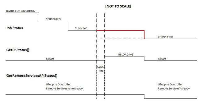
Figure 2 Typical Life Cycle of a 12G Configuration Job
