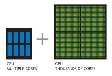
Figure 5 Number of cores in CPU vs. GPU [Source: NVIDIA]
