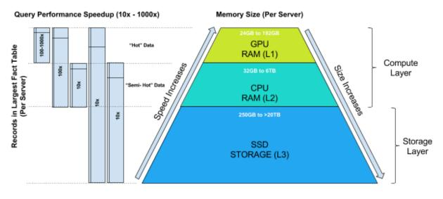
Figure 4 Query Performance with respect to IO bandwidth [Source: MapD]
