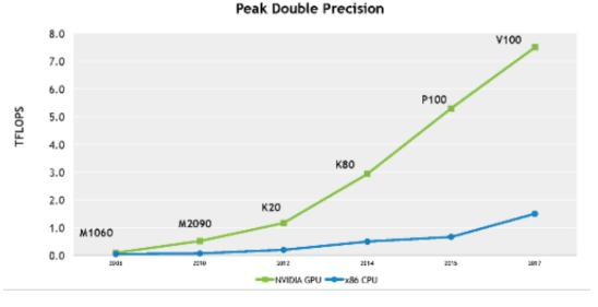
Figure 2 GPU Flop Comparison vs. CPU [source: NVIDIA]
