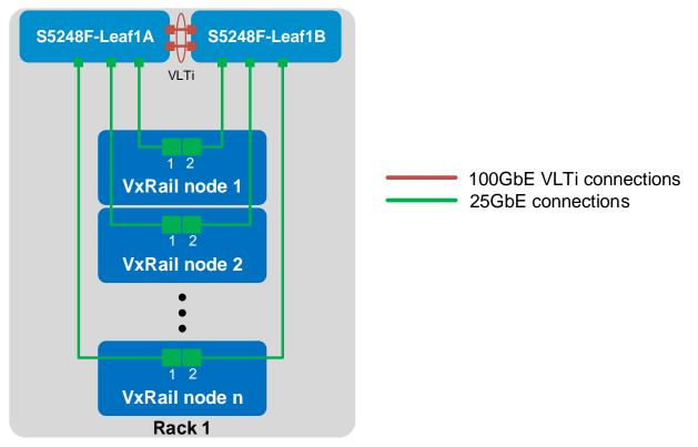
Figure 7 Dual switch topology with VLT
