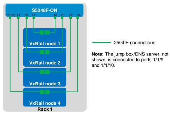
Figure 14 Four-node cluster connected to a single switch
