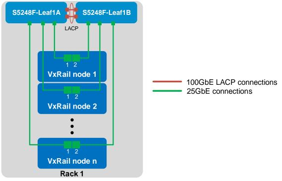
Figure 8 Dual switch topology without VLT
