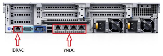
Figure 6 Rear view of VxRail 2-RU node (1-RU node is similar)
