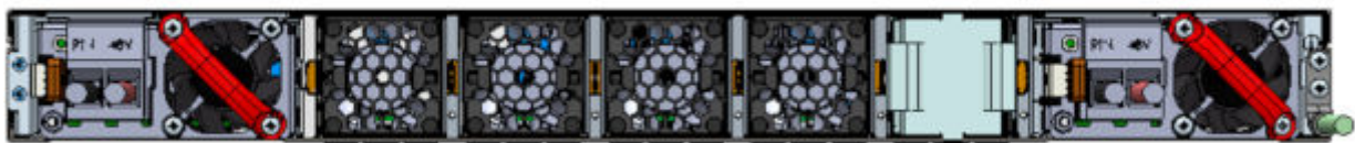
Figure 25. Installed DC PSU(s)
