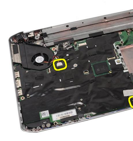
${\bf 23.}\,$  Remove the screws that secure the system board.
