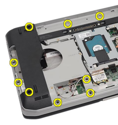
9. Flip the computer and remove the screws from the back of the computer.
