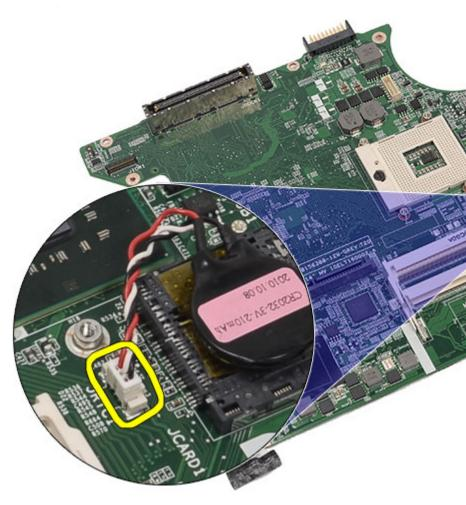
23. Pry and remove the coin-cell battery.
