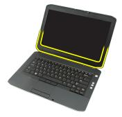
4. Work your way around the sides and the top edge of the display bezel.
