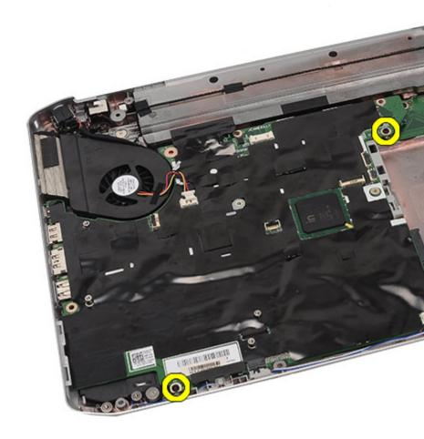
24. Lift the edge of the system board to disconnect it from the input/output  $(\mbox{I/O})$  panel.
