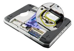
5. Remove the screw that secures the WLAN card to system board.
