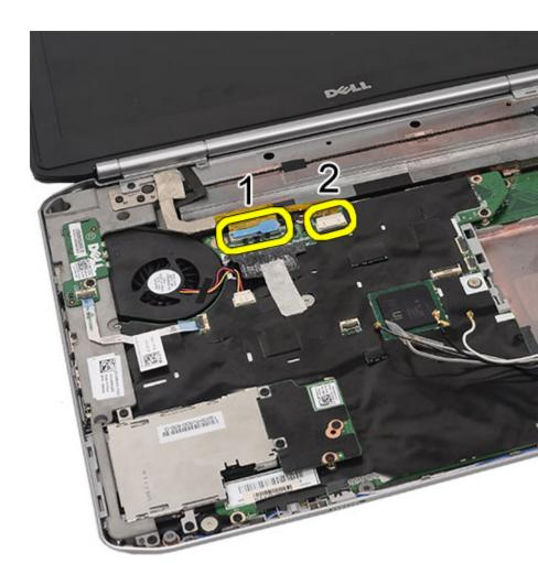
13. Remove the screws that secure the display assembly to the computer.
