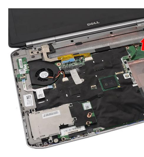
12. Disconnect the low-voltage differential (LVDS) and the camera cables.
