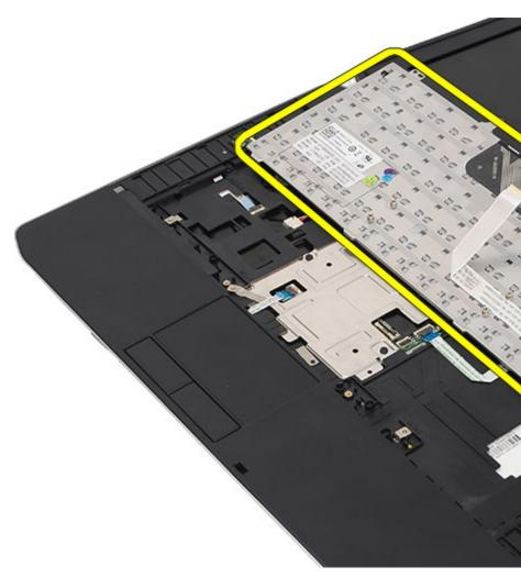
${\bf 9.} \quad \hbox{Disconnect and remove the cable from the keyboard}.$
