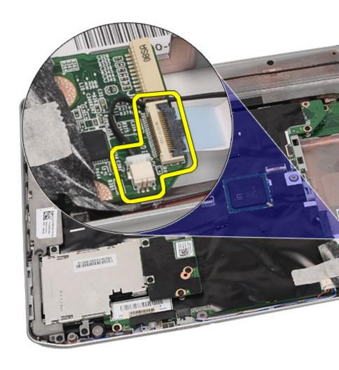
11. Remove the screw that secures the audio board to the computer.
