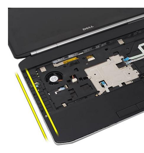
12. Release the tabs on the right edge of the palm rest assembly.
