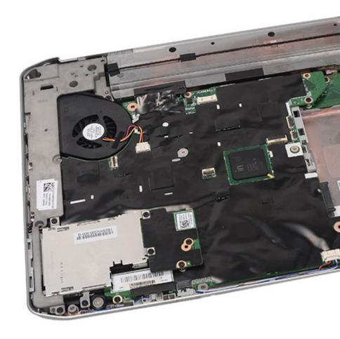
14. Disconnect the modem cable from the modem.
