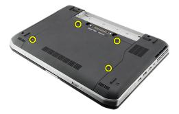
4. Slide and remove the back panel toward the front of the computer.
