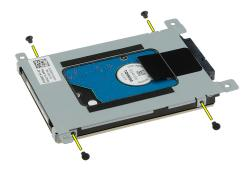
7. Disconnect the bracket from the hard drive.
