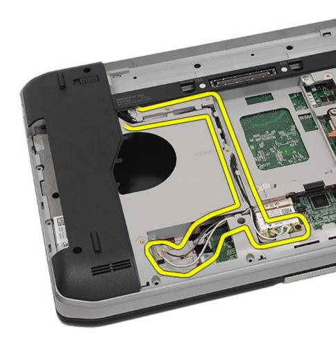
11. Remove the antenna cables from the routing channels.
