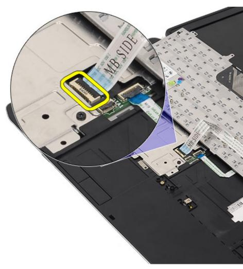
$8. \quad \text{Remove the keyboard from the computer}.$
