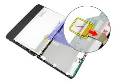
6. Remove the display panel from the display assembly.
