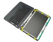
5. Disconnect the low-voltage differential signaling (LVDS) cable from the back of the display panel.
