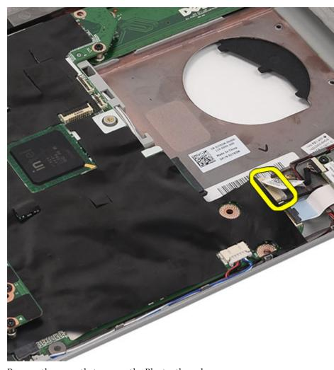
10. Remove the screw that secures the Bluetooth card.
