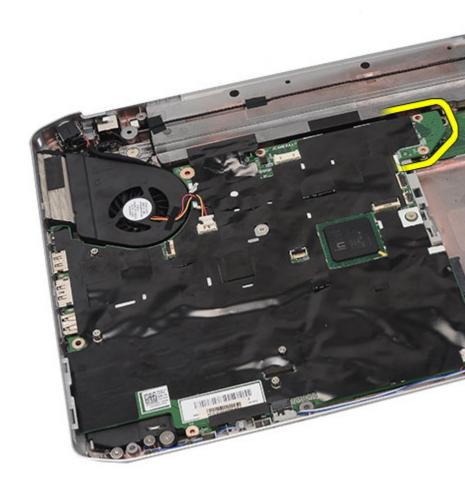
. Release the system board from the port connectors.
