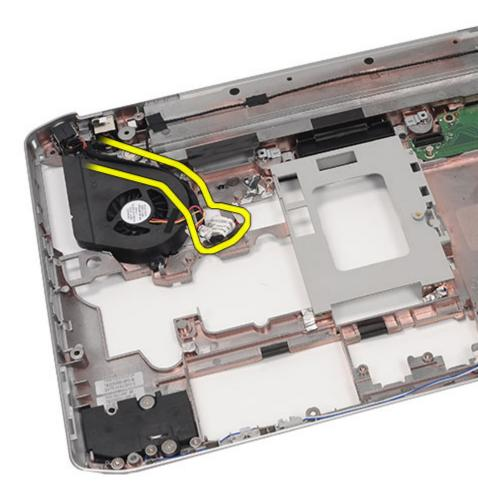
23. Remove the screw that secures the thermal fan.
