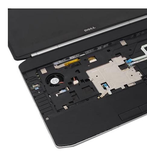
13. Remove the palm rest assembly from the computer.
