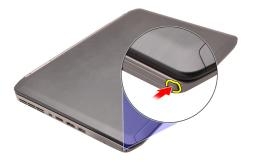
3. Press in on the PC latch to release the PC card.
