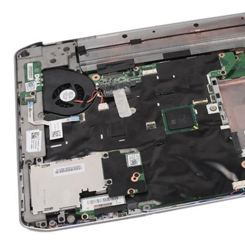
12. Remove the screws that secure the left support bracket.
