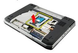
6. Remove the hard-drive bracket screws.
