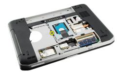
5. Push the screw tab away from the computer to release the optical drive from the drive bay.
