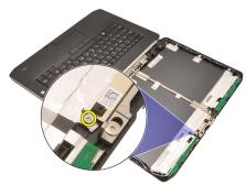
7. Lift and remove the camera module.
