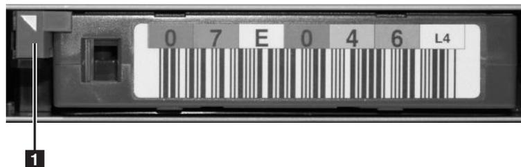
Figure 45. Cartridge release gate
