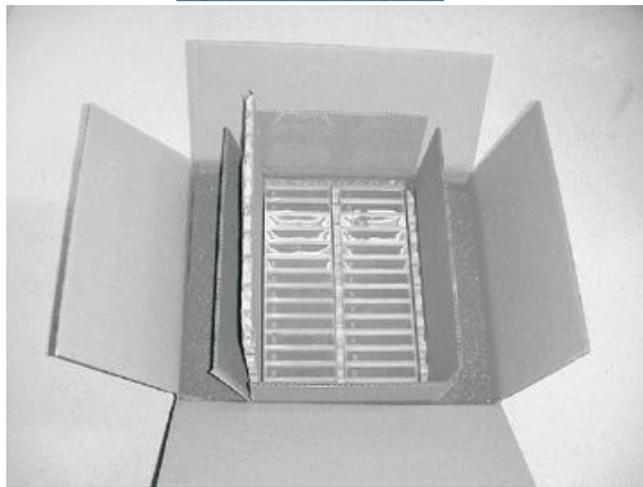
*Figure 111. Double-boxing tape cartridges for shipping*
