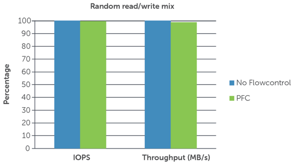
Figure 23 Random read/write I/O and throughput comparisons
