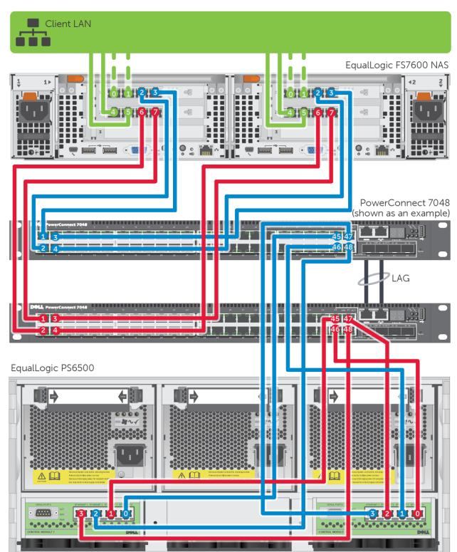
Figure 6 PowerConnect 7024 or 7048 with EqualLogic FS7600 and PS6500 (see Table 7 or Table 9).
