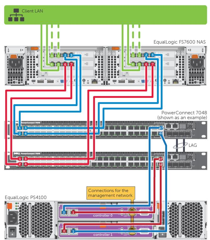
Figure 2 PowerConnect 7024 or 7048 with EqualLogic FS7600 and PS4100 (see Table 4 or Table 5).
