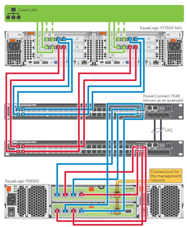
Figure 4 PowerConnect 7024 or 7048 with EqualLogic FS7600 and PS6100 (see Table 7 or Table 9).
