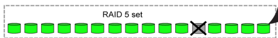
Figure 18 Surviving disk failures with RAID 5 as the member RAID level
