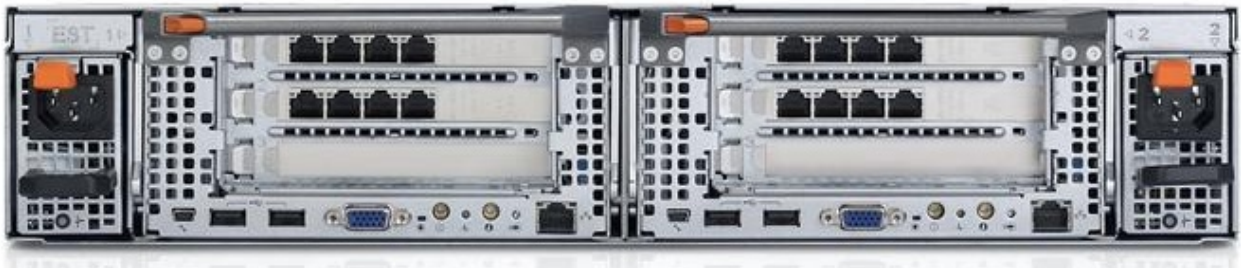
Figure 7 Rear view of FS7600 appliance showing network ports
