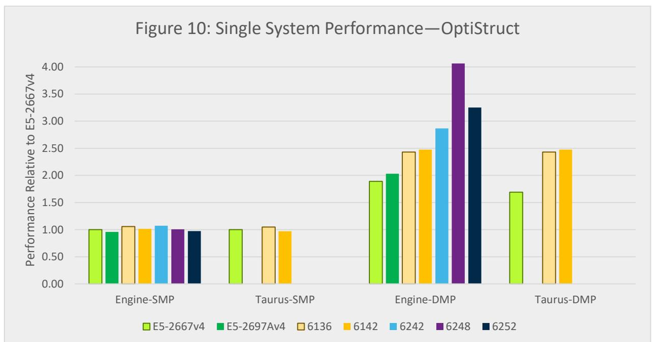
These results are shown relative to the performance of the 13G 8-core Intel Xeon E5-2667v4 based server, where higher indicates better overall performance. The E5-2667v4 based server had 512GB of memory with 2TB of local storage, the E5-2697Av4 server had 128GB of memory and 1TB of local storage, the 6136-based server had 384GB of memory and 2TB of disk space, and the remaining servers had 192GB of memory with 1TB of local storage.
