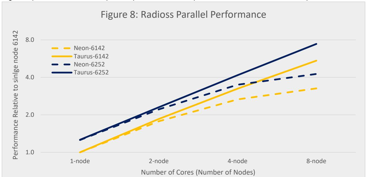
The figure uses the performance reference of 1.0 for a single node equipped with the Intel 6142. The overall parallel scalability for these models is good, behaving as expected, where the larger model shows better overall scalability. The single node performance improvement of the servers equipped with 6252 processors over the servers equipped with the 6142 processors is maintained for these benchmark runs up through eight nodes.
