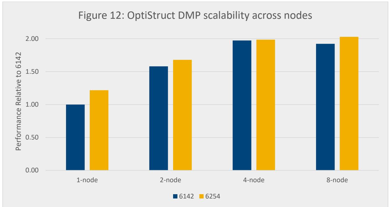
The reference for the plots was the single node 6142 server, where higher is better. One principle advantage of running OptiStruct jobs across nodes is that more memory and disk space is available when using multiple nodes, allowing larger models to be solved than could be solved using a single node. The results indicate good performance scalability when using multiple nodes.
