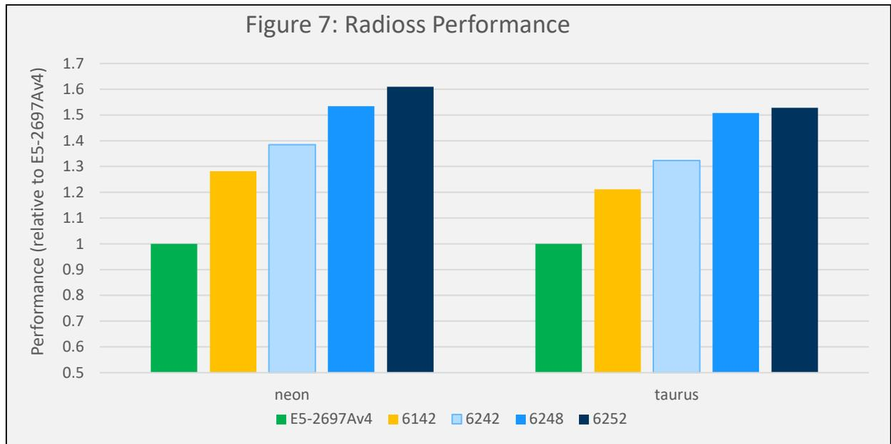
Here the performance is measured based on the elapsed solver time with the reference of 1.0 for the Dell EMC 13G Dell EMC R630 with dual Intel Xeon E5-2697Av4 16-core processors. The results are similar to the AcuSolve results, where the increase in performance from the 13G to the 14G servers is significant, particularly when 62xx series processors with a lot of cores are used.
