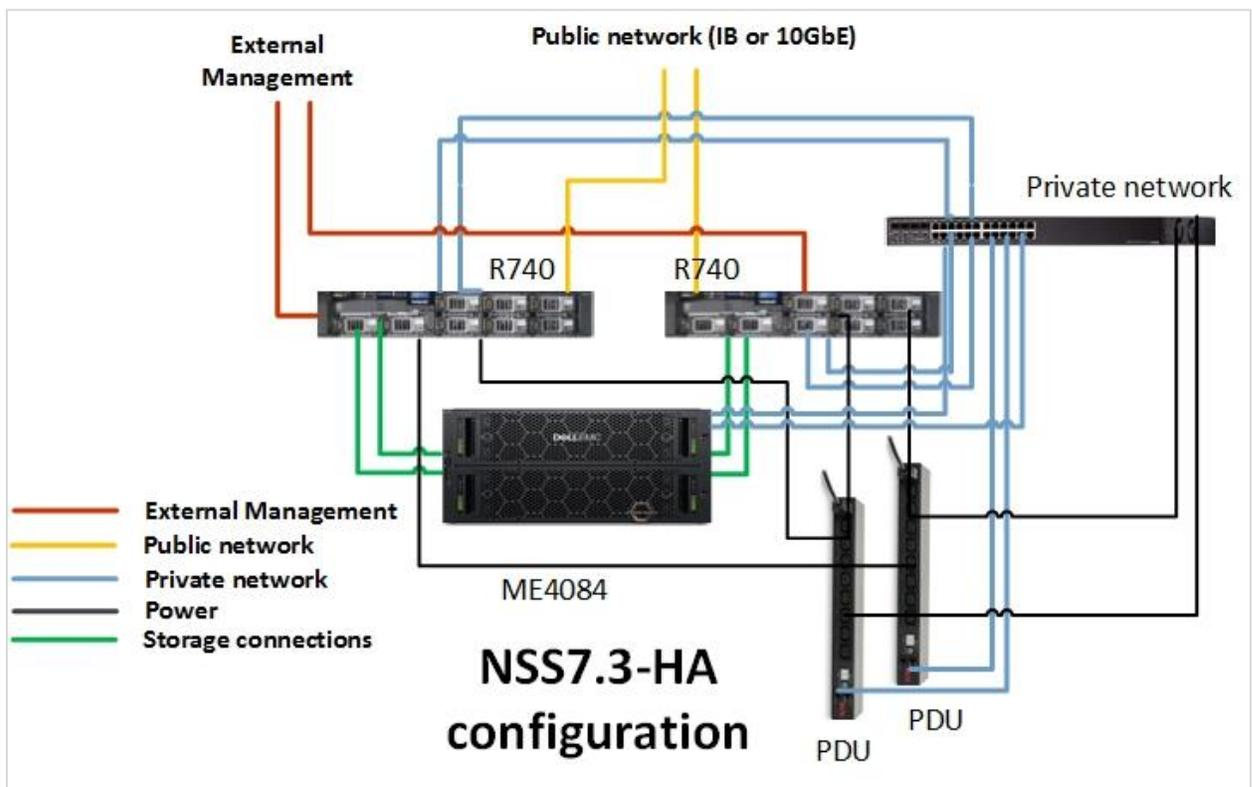
**Figure 2 NSS7.3-HA Storage System Architecture**
