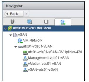
Figure 10 Completed distributed switch with port groups
