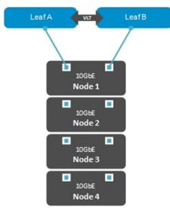
Figure 5 vSAN cluster using four server nodes connected to a leaf pair of switches
