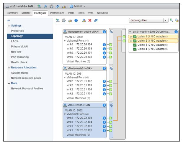
Figure 14 Final topology view for VDS with all port groups, VMkernel adapters, and uplinks configured
