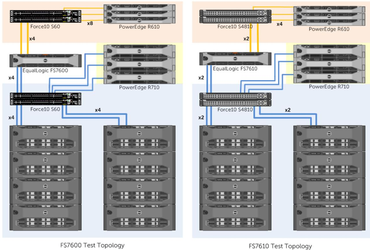
Figure 9 Test topology diagrams
