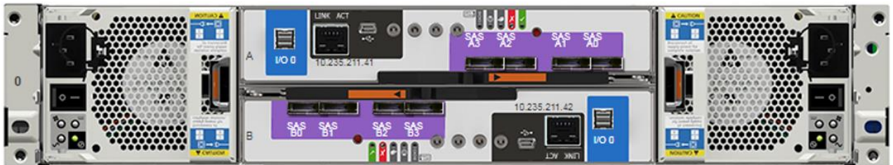
Figure 2 ME4 Series array with four SAS FE ports per controller
