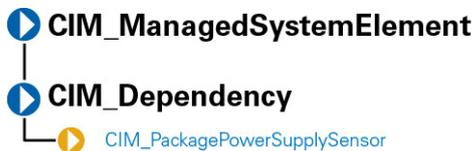
The `CIM_PackagePowerSupplySensor` class described in [CIM\\_PackagePowerSupplySensor Properties](#) contains power supplies that provide power to the whole package.
