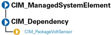
The `CIM_PackageVoltSensor` class described in [CIM\\_PackageVoltage Properties](#) contains voltage sensors that are often installed in a package such as a chassis or a rack to assist in the monitoring of the package in general. This relationship is described by the `CIM_PackageVoltSensor` association.
