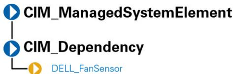
The DELL\_FanSensor class described in [DELL\\_FanSensor Properties](#) defines a Dell-specific association between a fan and a sensor. The CIM\_PackageFanSensor class contains fans that assist in cooling the entire package as opposed to a fan dedicated to cooling only some of the components in the package.
