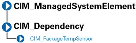
The `CIM_PackageTempSensor` class described in [CIM\\_PackageTempSensor Properties](#) contains temperature sensors that are often installed in a package such as a chassis or a rack to assist in the monitoring of the package in general. This relationship is described by the `CIM_PackageTempSensor` association.
