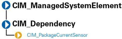
The `CIM_PackageCurrentSensor` class described in [CIM\\_PackageCurrentSensor Properties](#) contains amperage sensors that are often installed in a package such as a chassis or a rack to assist in the monitoring of the package in general. This relationship is described by the `CIM_PackageCurrentSensor` association.
