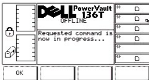
Abbildung 54. Dialogfeld "Command" > "Drives" > "Unload" > "Command in Progress"
