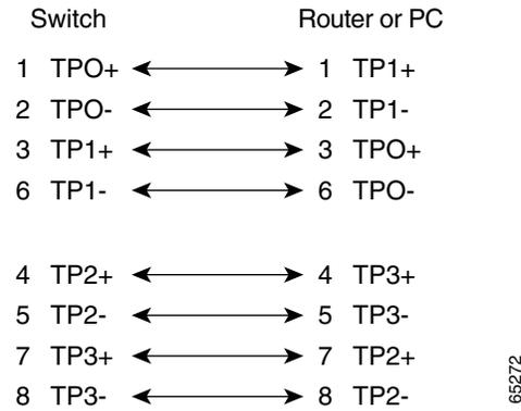
**Figure B-9** Four Twisted-Pair Crossover Cable Schematics for 10/100/1000 Ports
