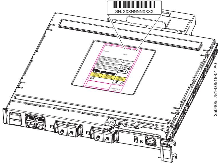
**Figure 3-2** Serial Number Location on the Cisco Catalyst Blade Switch 3032 for Dell
