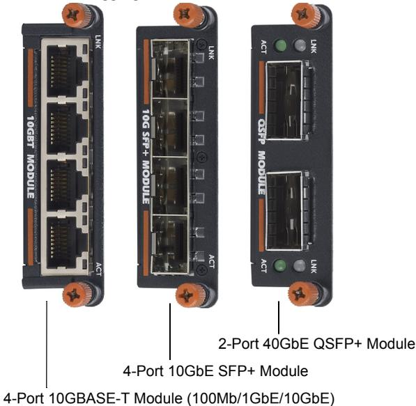
Use the FlexIO modules in an Aggregator that operates in standalone or stacking mode:
