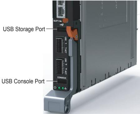
Use the lower USB console port (Figure 1-3) to manage the switch through an RS-232 serial interface. This port provides a direct connection to the switch and allows you to access the command-line interface (CLI) from a console terminal connected to the port through the provided serial cable (with USB type-A to female DB-9 connectors).
