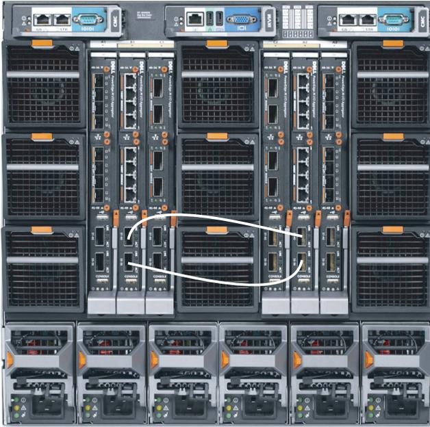
Use only QSFP transceivers and QSFP cables (separately purchased) to connect stacking ports; for example:
