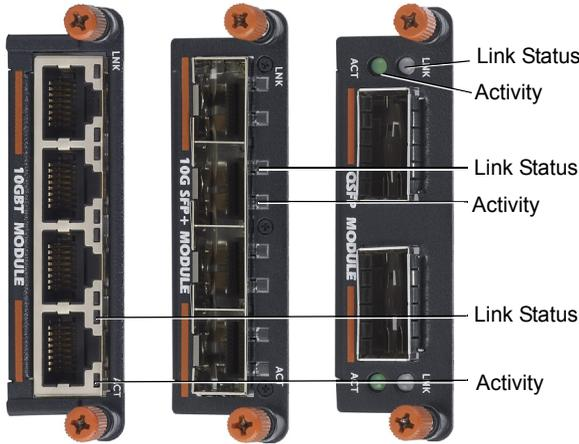
Table 1-2 describes the LED status of 10GbE BASE-T, 10GbE SFP+, and 40GbE QSFP+ ports used in stacking mode on the base module.
