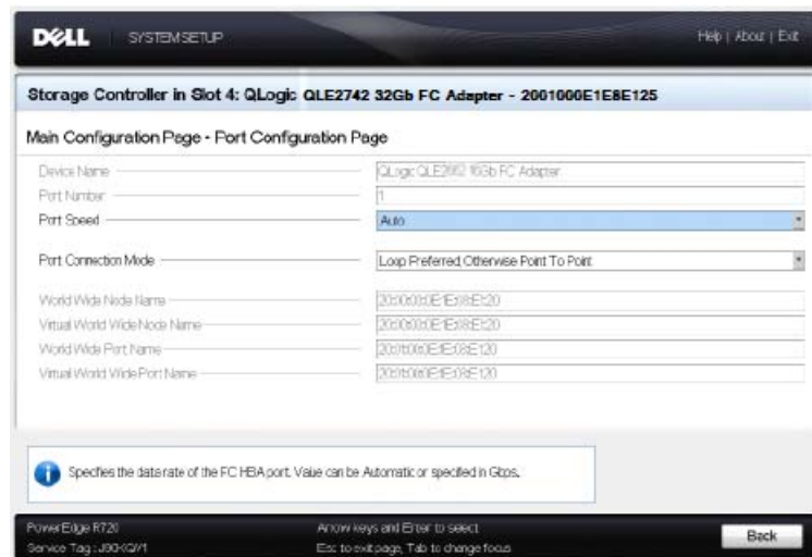
Figure 3-13. Dell System Setup: Port Configuration
