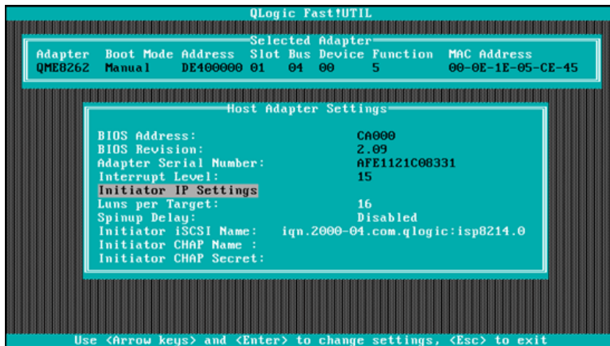
Figure 5-23. Fast!UTIL: Host Adapter Settings Window
