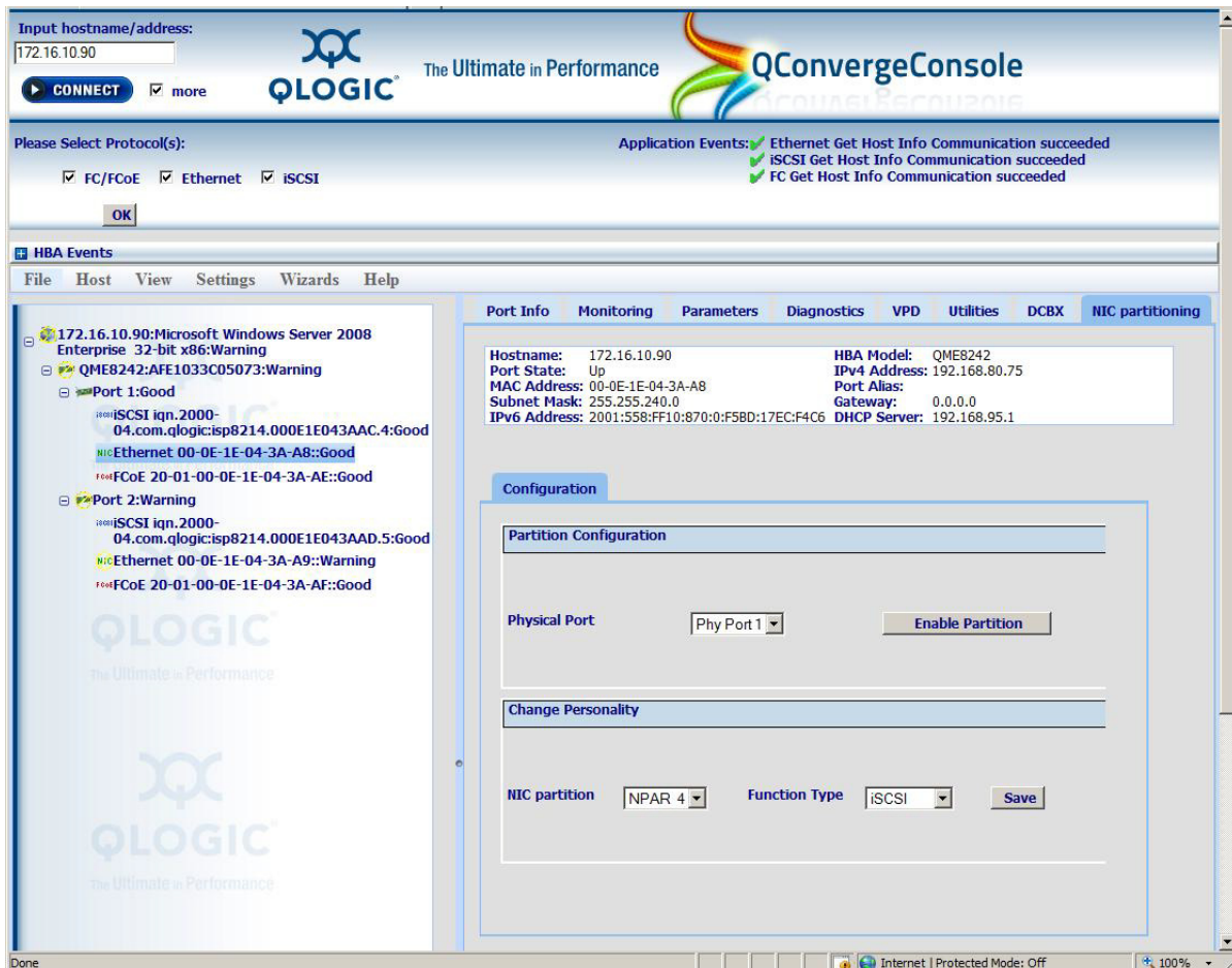
Figure 4-15. NIC Partitioning (Switch Independent Partitioning) Configuration Page
