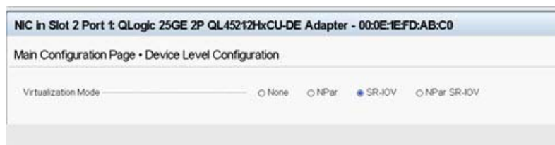
Figure 8-2. System Setup for SR-IOV: Device Level Configuration
