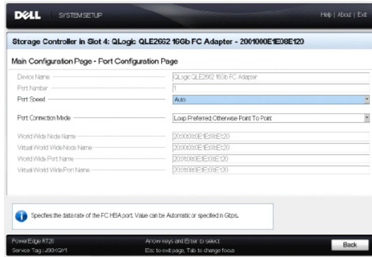
Figure 3-13. Dell System Setup: Port Configuration
