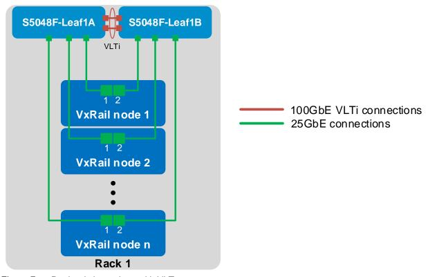
Figure 7 Dual switch topology with VLT
