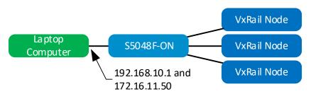
Figure 15 Use of a laptop computer for deployment
