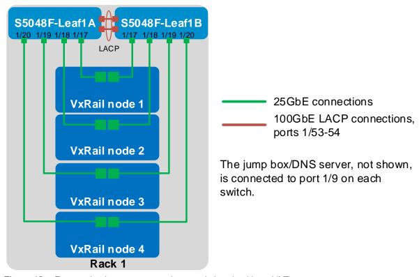
Figure 13 Four-node cluster connected to a switch pair without VLT
