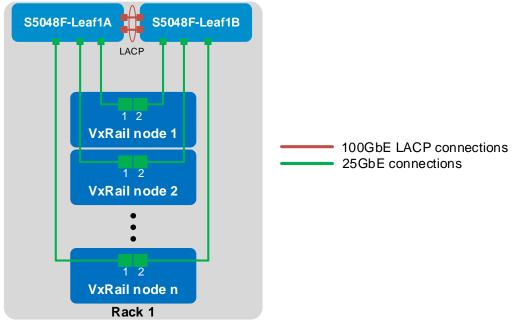
Figure 8 Dual switch topology without VLT
