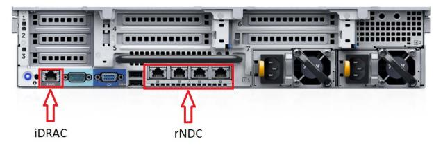
Figure 6 Rear view of VxRail 2-RU node (1-RU node is similar)
