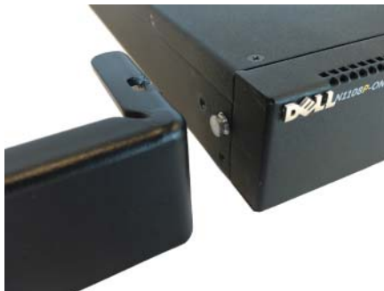
Figure 1-6. Attaching the Brackets
