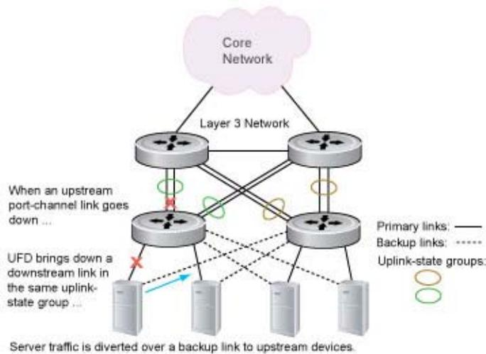
If only one of the upstream interfaces in an uplink-state group goes down, a specified number of downstream ports associated with the upstream interface are put into a link-down state. This number is user-configurable and is calculated by the ratio of upstream port bandwidth to downstream port bandwidth in the same uplink-state group. This calculation ensures that there are no traffic drops due to insufficient bandwidth on the upstream links to the routers/switches.
