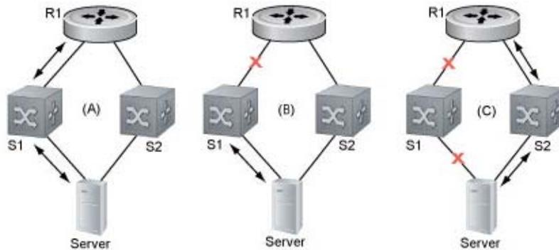
A: Switches 1 and 2 have upstream and downstream connections to Router1 and Server via primary links.
