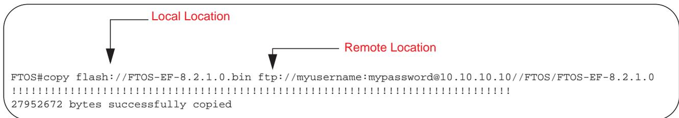
Figure 4-10 shows an example of using the copy command to import a file to the Dell Force10 system from an FTP server.
