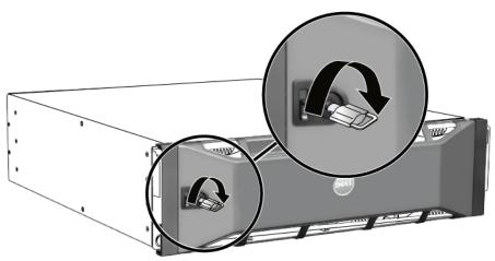
Figure 2-3: Unlocking the Bezel
