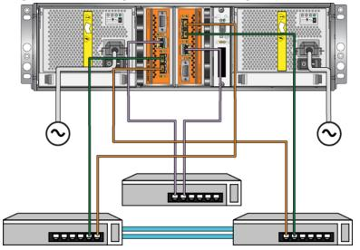
Figure 3-11: Configuration With Management Network
