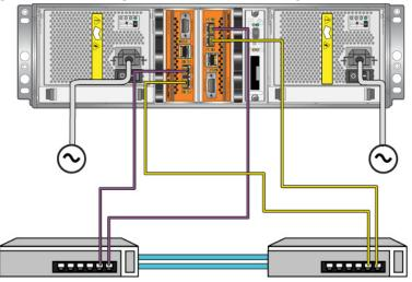
Figure 3-10: Configuration Without Management Network)
