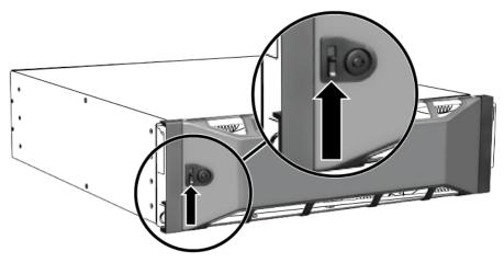
Figure 2-4: Pushing Up the Bezel Release Latch
