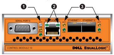
Figure 3-1: Type 10 Control Module
