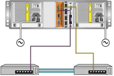
For a dual control module array, at a minimum, connect network cables to Ethernet 0 on both control modules and then connect the cables to a network switch. See Figure 3-9.
