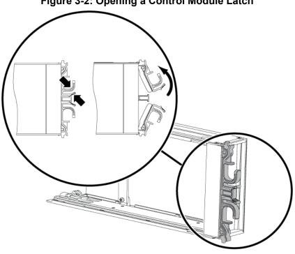
2. Hold the latches and carefully slide the control module from the slot. See Figure 3-3.
