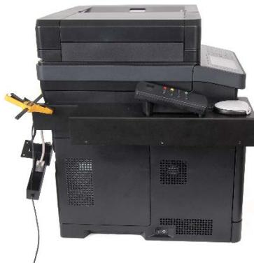
Connect the CACStar Ethernet cable to the S2815 Ethernet port. Use the three supplied screws to attach the back assembly to the S2815. Use the M3 x 50mm screw for the lower hole to attach the CACStar using the hole from which the screw was removed earlier. Do not overtighten this screw. Use the 2 M3 x 10mm screws for the upper holes to attach the back assembly to the base CACStar assembly as shown below.
