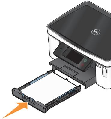
**Note:** If you extended the tray to accommodate A4- or legal-size paper, then the tray sticks out from the front of the printer when inserted.
