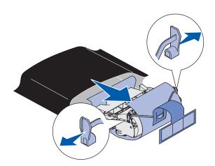
**NOTICE:** Do not touch the photoconductor drum on the underside of the toner cartridge.
