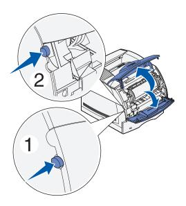
Press down on the side door latches and open the side door.
