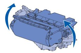
2 Align the arrows on either side of the toner cartridge with the corresponding arrows in the printer.
