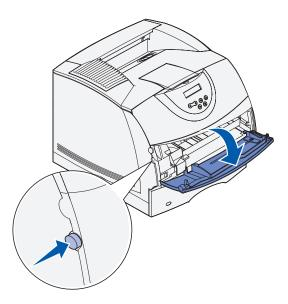
2 Locate the metal bar in the recessed area on the multipurpose feeder. Pull the bar out far enough to accommodate the print media you will be using.
