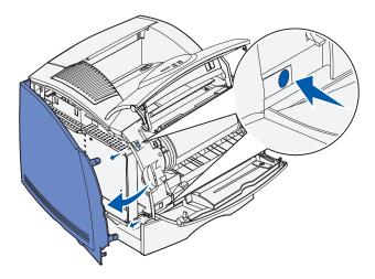
Use a small Phillips screwdriver to loosen, but not remove, the six screws on the shield.
