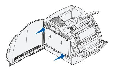
**5** Use the tabs to slide the shield up until the top three screws fit into the three keyholes on the shield.
