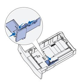
**3** Squeeze the length guide lever and slide the length guide to the correct position for the size of print media you are loading.
