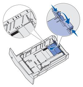
Before loading print media, flex the sheets back and forth to loosen them, and then fan them. Do not fold or crease the print media. Straighten the edges of the stack on a level surface.
