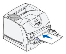
**6** Slide the width guide to the left until it lightly touches the stack of print media. *Do* not bend the print media.
