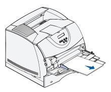
2 Push the metal bar straight back to collapse the multipurpose feeder to its short-length position.
