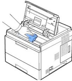
CAUTION: While cleaning the inside of the printer, be careful not to touch the transfer roller located underneath the toner cartridge. Oil from your fingers can cause print quality problems.
